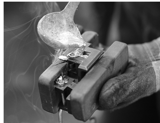
Manual casting of lead type in the museum
